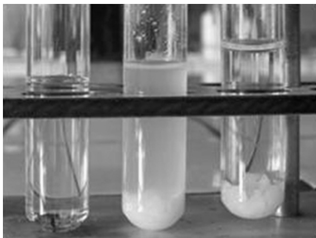
Fig. 2. Pictures of PCL solubility states. From left to right: soluble (a), partially soluble (b) and non-soluble (c).
